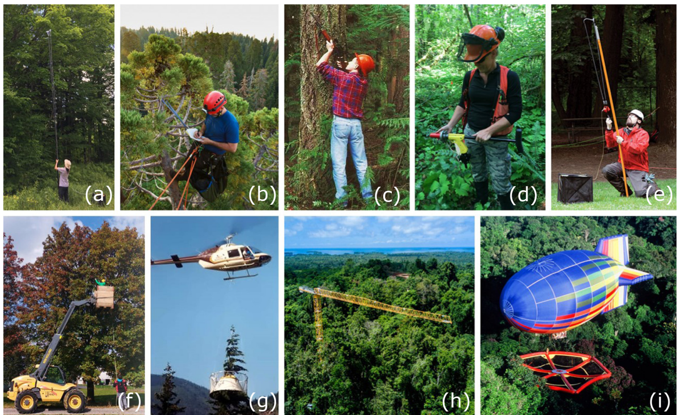
Fig. 2: Current practices for tree sampling [1]: (a) pole pruner [2] – a long pole to collect leaf samples; (b) climber [2] – climbing on top of a giant sequoia which is one of the largest trees (220 feet) with ropes; (c) shotgun [3] – collecting by shooting cone-bearing branches from a tree; (d) line launcher [4] – setting up the tree climbing rope lines; (e) slingshot [4] – line launcher with throwing the weights; (f) hydraulic lift [5] – fork-lift sampling at various heights up to 8m; (g) helicopter [3] – collecting cones by helicopter requires additional safety equipment; (h) canopy crane [6] – tower crane built in the middle of the forest; (i) canopy raft [7] – a huge net supported by an airship and designed to be landed on the canopy.
