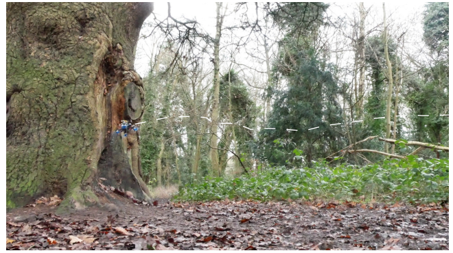
Fig. 9: BeeMAV: a palm-sized drone with a total weight of 158 g [32]. The platform utilizes two optical flow sensors to trigger safety actions for collision avoidance.
