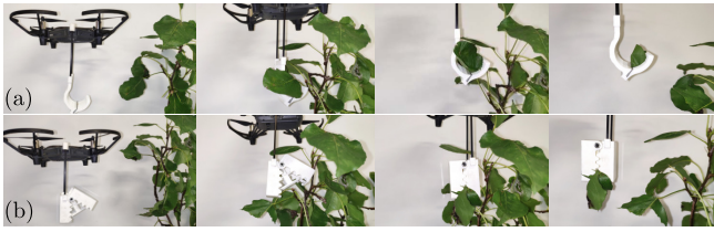
Fig. 7: Small drone for leaf sampling (from left to right) - (a) comb-like mechanism attached from the bottom; (b) passive trap-like mechanism for the sample collection from top.
