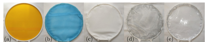
Fig. 6: Materials for basket mechanism: (a) sticky paper; (b) polypropylene; (c) PUL fabric; (d) fabric net; (e) PVC.
